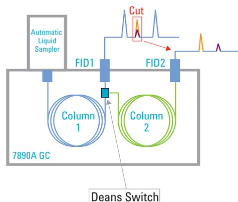
In this example, the Capillary Flow Deans Switch provides additional selectivity that enables the analysis of unresolved trace components by heart-cutting onto another column having a different stationary phase.
