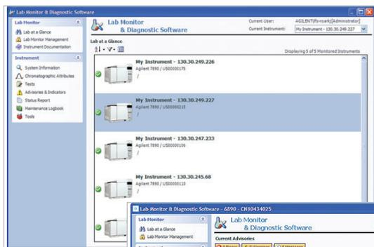
**Lab-at-a-Glance feature** lets you view the operational status and maintenance needs of a single system or multiple systems lab-wide.
