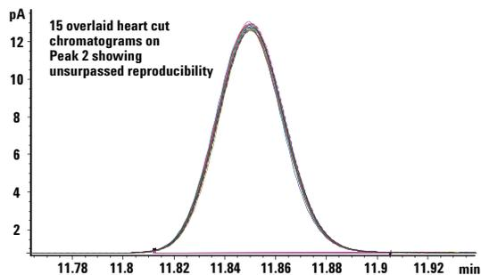
Not only is one ensured unsurpassed retention time reproducibility in standard applications, but also in multi-dimensional applications such as the heart-cutting example shown here.
