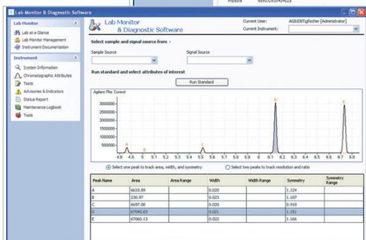
**It even keeps an eye on the results.** You can also have the software alert you to perform inlet and/or column maintenance when specified chromatographic attributes fall outside preset windows—without the need for subjective interpretation or the intervention of a highly skilled chemist.
