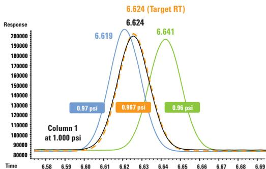
5th-generation EPC and advanced digital electronics set a new benchmark in pressure setpoint precision (to 0.001 psi)—improving RTL precision for very-low-pressure applications.
