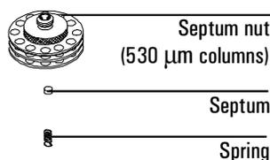
4. Insert the narrow wire (or a piece of capillary column) into the inlet through the oven, and push the insert and spring (if they did not come out previously) out through the top of the inlet.
