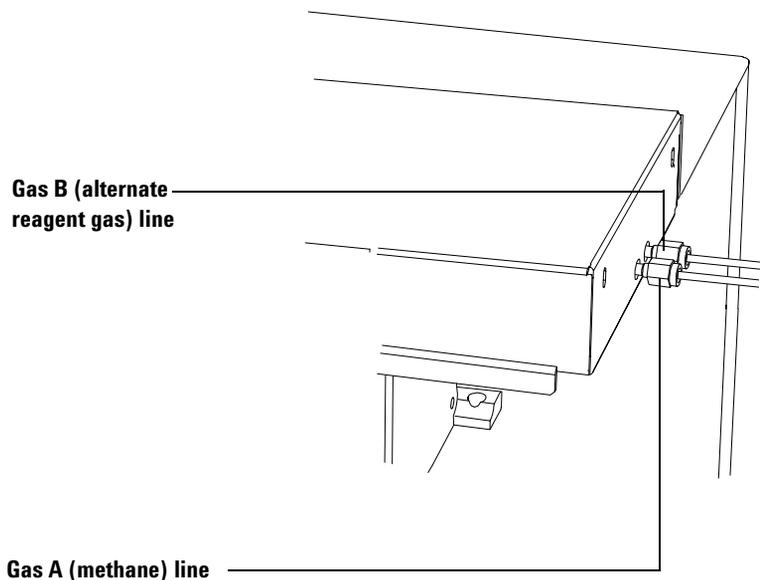
**Figure 6** Connecting the methane line
