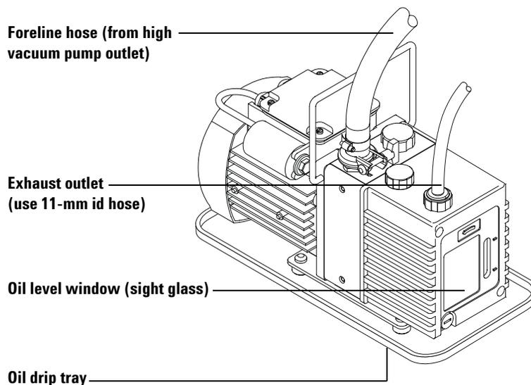
**Figure 5** Preparing the vacuum system
