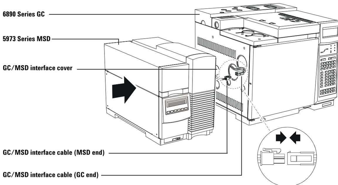
**Figure 7** Connecting the MSD and the GC
