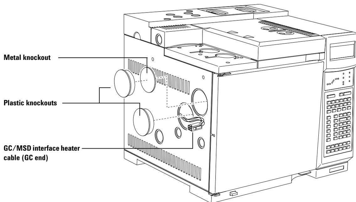
**Figure 3** Removing the knockouts
