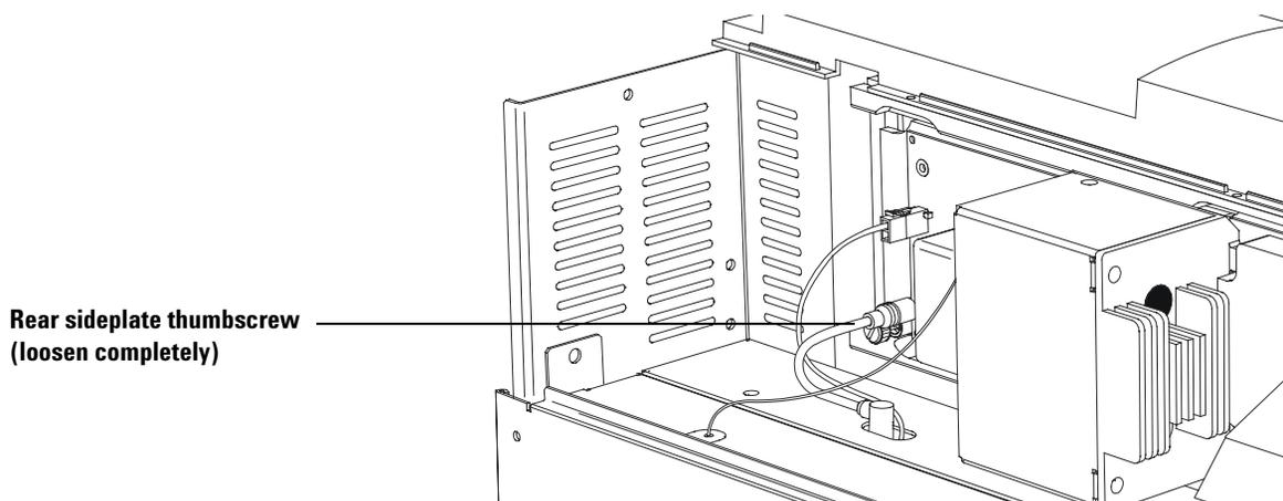
**Figure 8** Loosen sideplate thumbscrews
