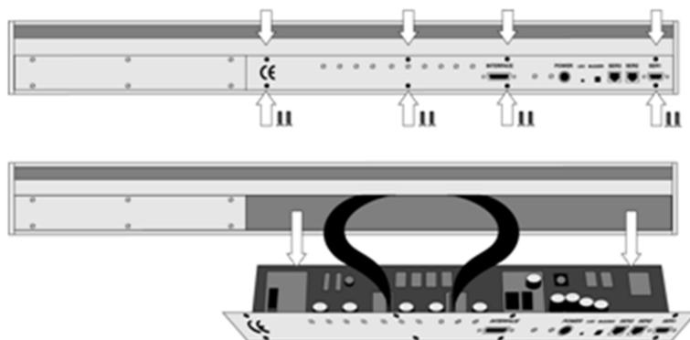
Figure 45. Replacing Control-GC Board
