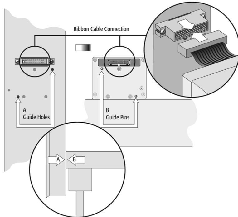
**Figure 11.** Connecting the Injection Unit Ribbon Cable
