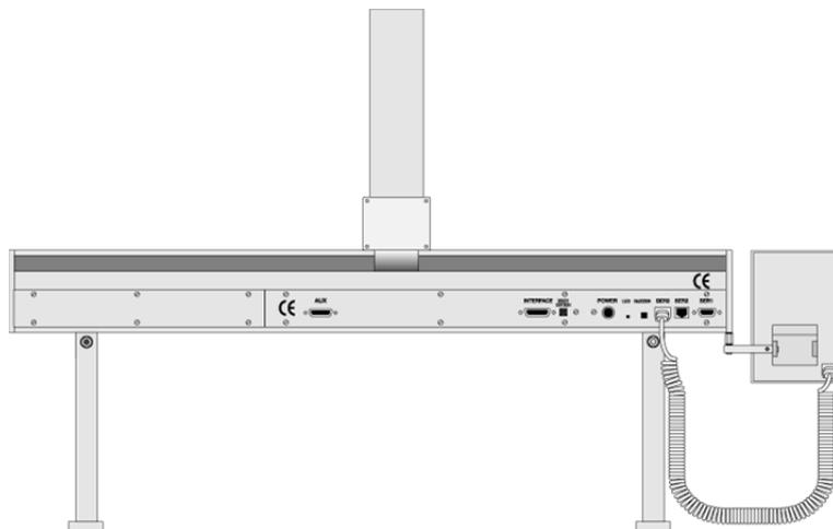
**Figure 17.** Electrical Connections for GC PAL System
