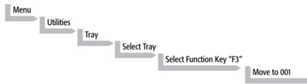
A dialog window opens, displaying a note to “Adjust offset X-, Y-, Z for position 001”. Continuing in this dialog will provide the user the opportunity to adjust all three axes perfectly by the top of the vial. Please note that this step is only valid for position number 001.
