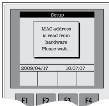
**Figure 37.** Reading the MAC Address from the Ethernet Communication Port
