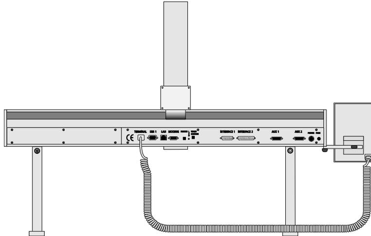
Figure 18. Electrical Connections to PAL GC-xt System
