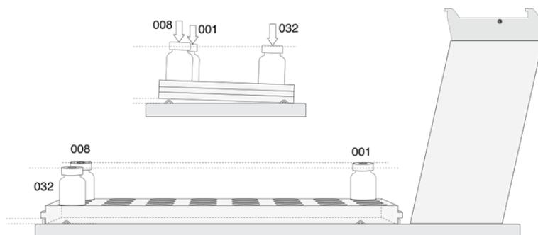
Figure 23. Demonstrating a possible Inclination of Tray in X-,Y-,Z-Axes.
