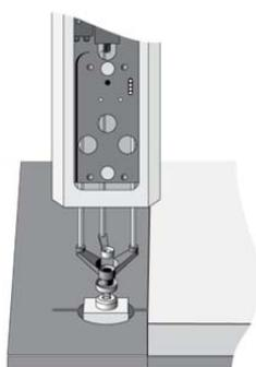
Figure 33. GC Injectors (e.g. GC Inj1) Reference Position
