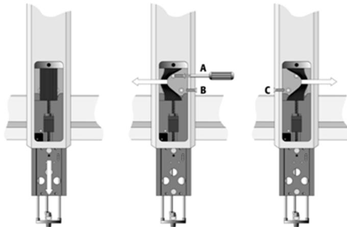
**Figure 12.** Inserting the Injection Unit Mounting Torx Screws
