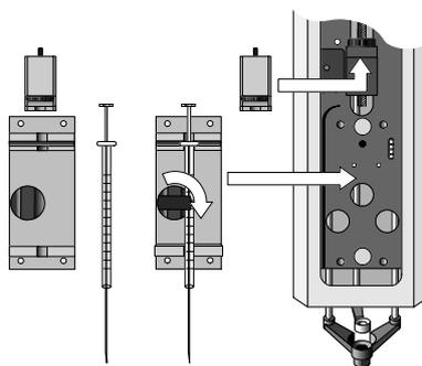
**Figure 34.** Syringe and Syringe Adapter for Liquid Injections
