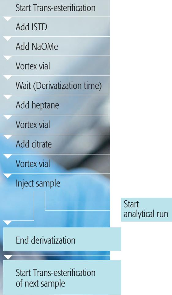
The trans-esterification of fatty acids to generate the corresponding methyl esters (FAME) is a very common and at the same time tedious procedure. Its automation increases productivity and prevents exposure of humans to hazardous chemicals.
