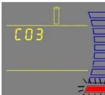
**NOTE: The lowest water level is not calibrated if the amount of water emptied from the tank is less than 10%.**
