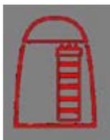
When the red Pack Alarm is displayed as a steady icon, the SimpliPak cartridge is not installed correctly or not installed at all. If the SimpliPak cartridge has been reinstalled and the Alarm is still displayed, then contact Millipore.
