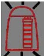
The system will prompt you to change the SimpliPak cartridge using a red Pack Alarm icon. The Display will show the red Pack Alarm blinking. The SimpliPak cartridge is changed due to either the amount of time it has been used or from the amount of water that has passed through it.
