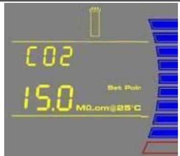
3. Press the "+" or "-" Button to adjust the Resistivity Setpoint from 1.0 M $\Omega$ .cm @25 °C to 18.0 M $\Omega$ .cm @25 °C.
