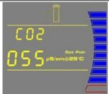
If Conductivity Units are chosen in C01, then the Setpoint can be adjusted from 0.999  $\mu$ S/cm @25 °C to 0.055  $\mu$ S/cm @25 °C.
