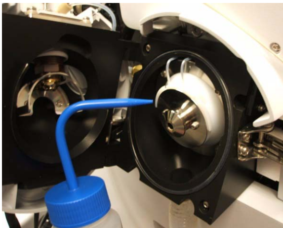
Figure 20 Rinsing the area around the spray shield
