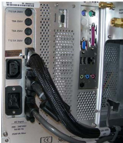
Figure 75 Disconnect the instrument power cable.
