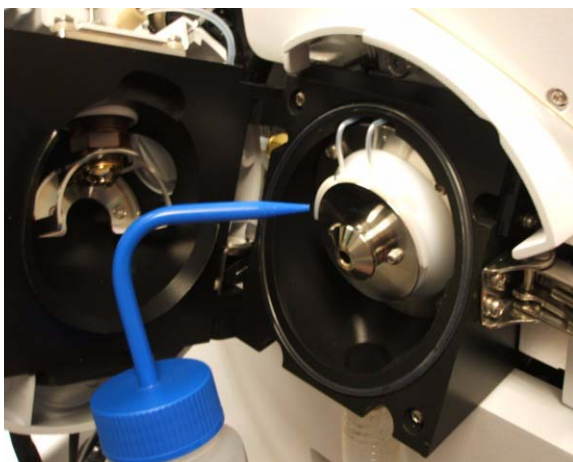
Figure 9 Rinsing the area around the spray shield
