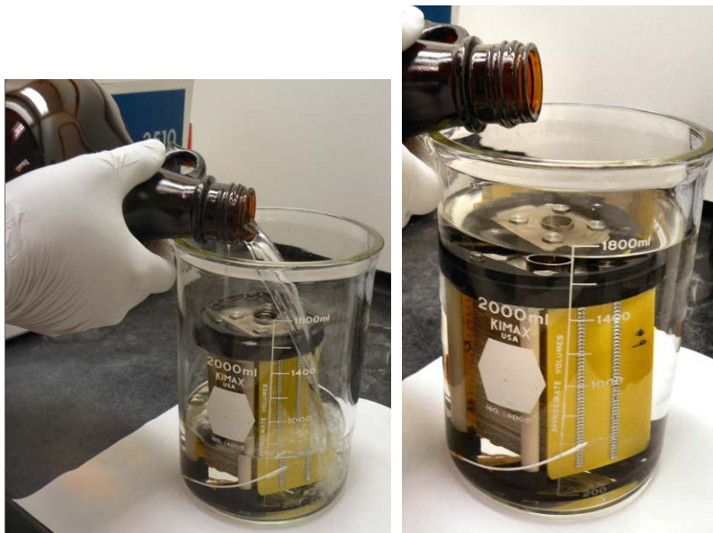
Figure 69 Pouring isopropanol into the glass beaker.
