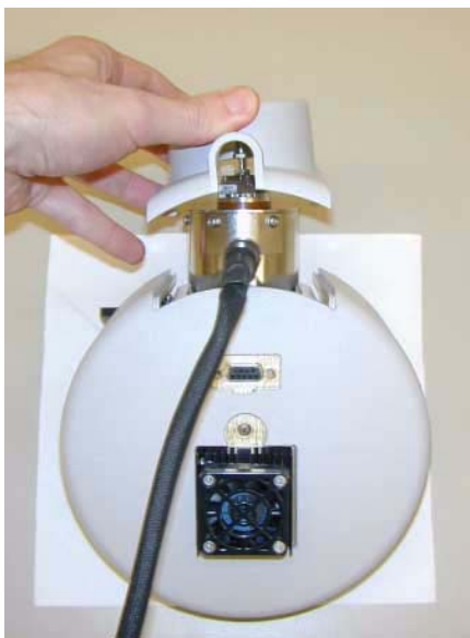
Figure 38 Removing the Nebulizer Cover (left) and Removing the Cosmetic Cover screws
