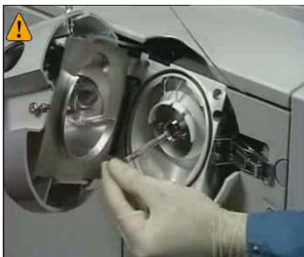
Figure 50 Reinstalling the capillary
