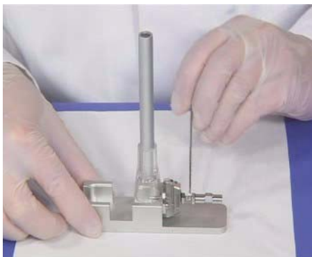
Figure 32 Installing the nebulizer in the adjustment fixture
