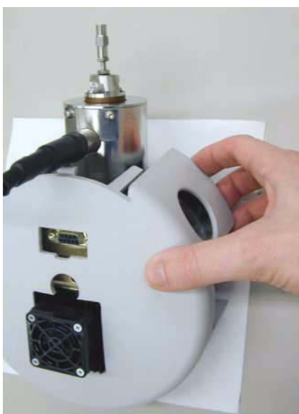
Figure 39 Removing the Cosmetic Cover
