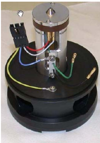
Figure 64 The re-assembled ion optics assembly
