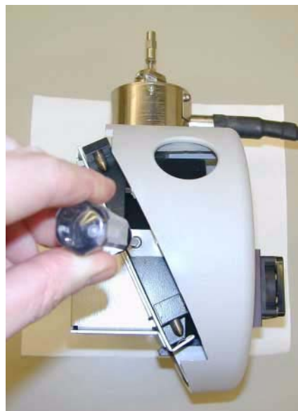
Figure 38 Removing the Nebulizer Cover (left) and Removing the Cosmetic Cover screws
