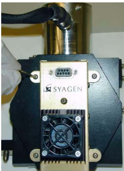
Figure 40 Use a 2 mm Hex Key (left) and Nylon Insulators
