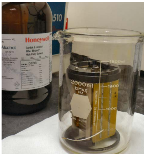
Figure 68 High Pressure Ion Funnel in a glass beaker.
