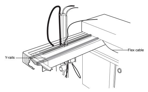
5. Wipe the inside of the flex cable channel using a lint-free cloth dampened with isopropyl alcohol.
