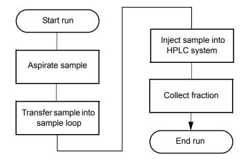
The hardware components move the sample as follows:
