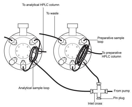
12. Reposition the inject valve and tighten the mounting clips.
