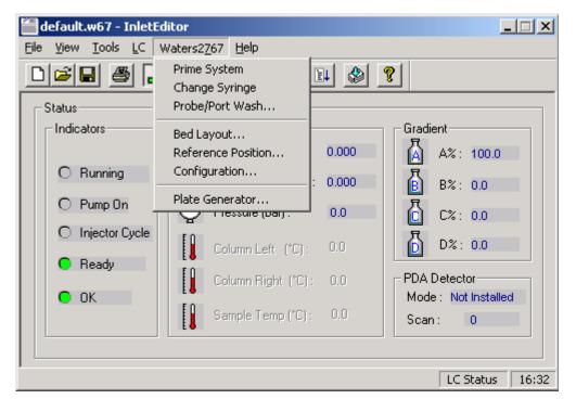
If you selected two wash solvents from the Configuration dialog box, the wash pump is primed sequentially with wash solvent 2, then wash solvent 1. The prime system cycle moves the sample probe to the wash station and primes the wash pump, then draws the wash solvent into the syringe. The wash solvent rinses the inner and outer surfaces of the sample probe. The priming sequence stops automatically and the sample probe returns to the home position.
