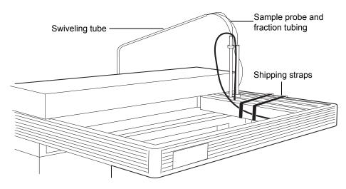
2. Remove the packing material from the top of the frame. Remove the tie wrap and tubing from the top of the probe guide, and remove the tie wrap from the probe below the frame.
