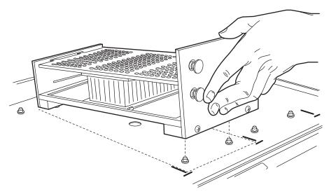
Gilson<sup>®</sup> racks can be used for fraction collection. When placing such racks on the worktable, use the small, circular marks to position the curved front of the rack.
