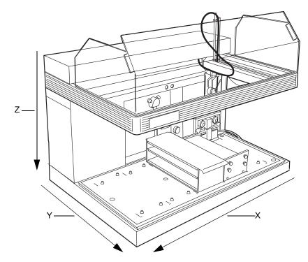
3. Click the Adjust Coordinates screen or use the arrow keys (right and left for X-direction, up and down for Y direction, or Page Up and Page Down for Z direction) to move the sample probe to the top of the reference button. Select an arm speed appropriate for the amount of movement required.
