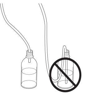
4. Secure the tube to the container. Loosely cover the waste container opening with laboratory film to prevent fumes and splashes without sealing it tightly.
