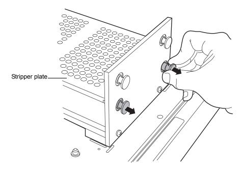
2. Lift the front of the stripper plate up over the front of the rack, and then slide the stripper plate toward the front to dislodge the back of the stripper plate from the rack.
