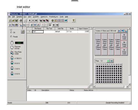
The Inlet Editor controls the each component of the AutoPurification System. To access the 2767 Sample Manager method parameters, click from the
