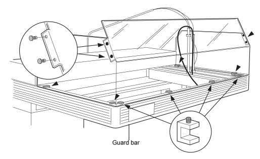
3. Place the four shield clips with the set screws facing upward onto the flange in the notches. Use an Allen wrench to tighten the set screw in the clamp.
