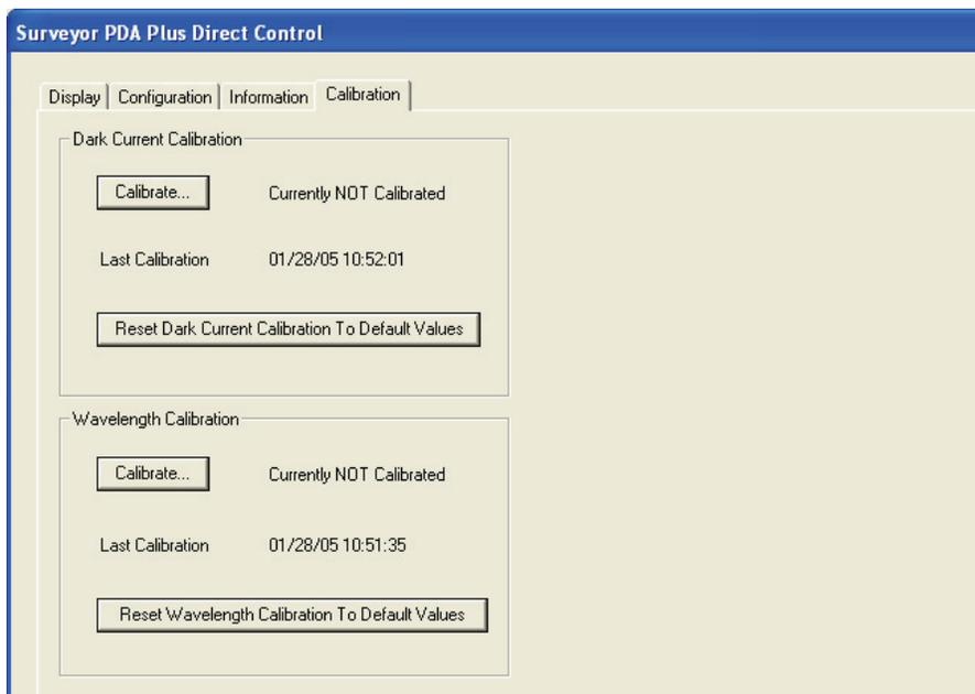
**Figure 58.** Calibration page, showing that the detector is currently Not calibrated
