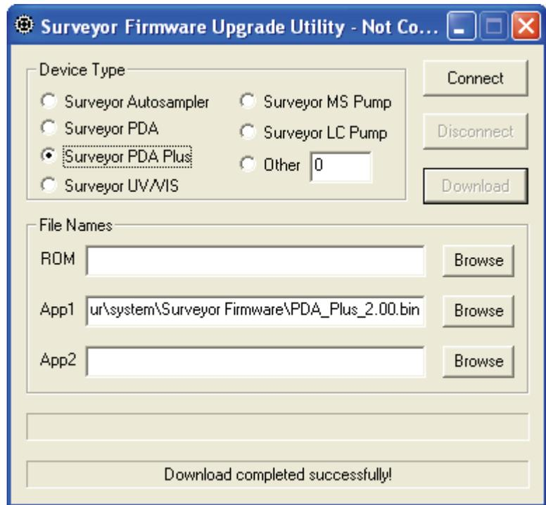
**Figure 87.** Surveyor Firmware Upgrade Utility, showing the PDA\_Plus\_\*.bin file selected
