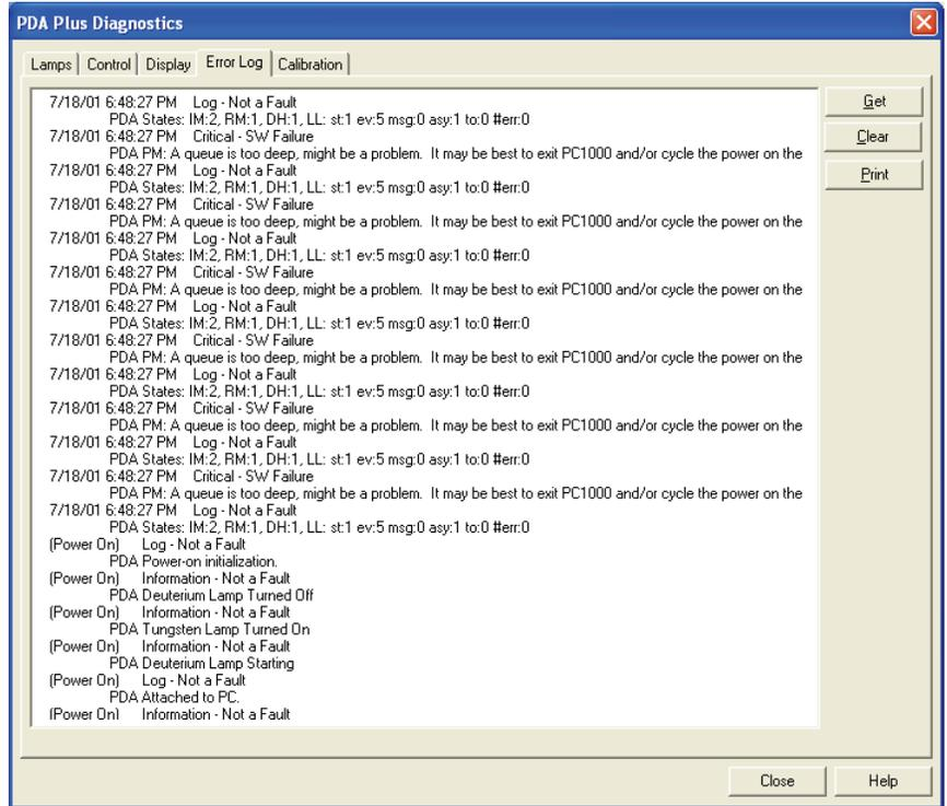
**Figure 37.** PDA Plus Diagnostics dialog box, showing the Error Log page
