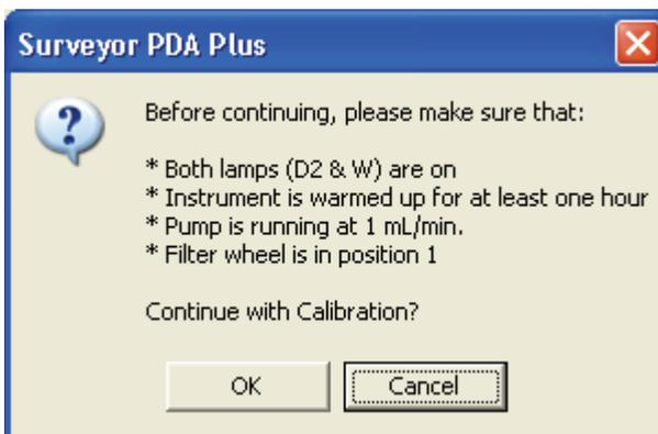
**Figure 32.** Calibration Preconditions
