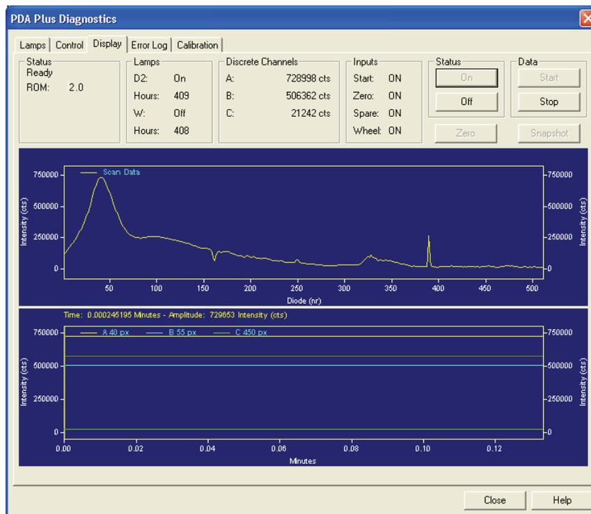
**Figure 39.** PDA Plus Diagnostics dialog box - Display page, showing an intensity scan with the deuterium lamp
