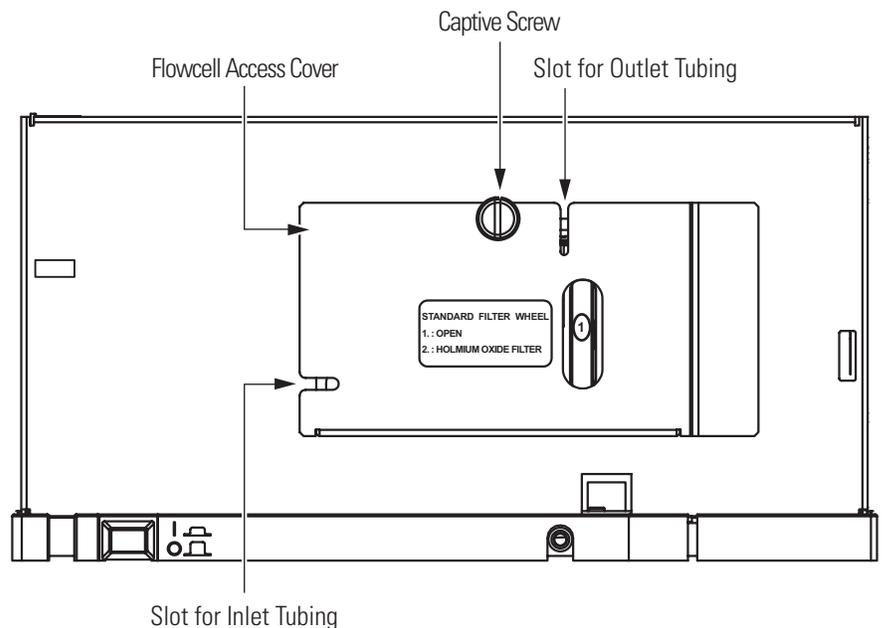
**Figure 13.** Surveyor PDA Plus Detector with doors open, showing the flow cell access cover
