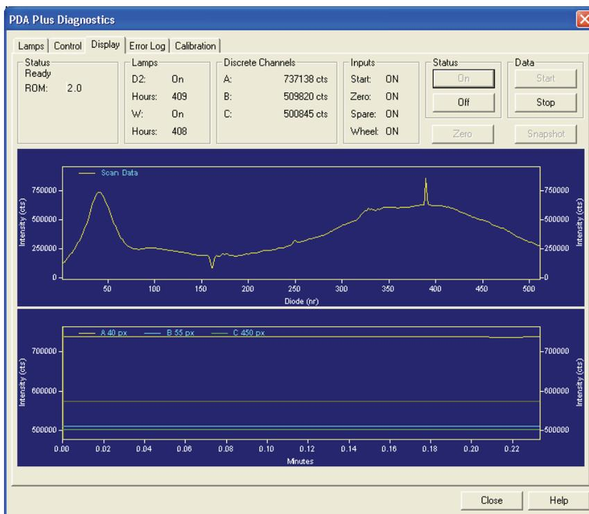
**Figure 40.** PDA Plus Diagnostics dialog box – Display page, showing an intensity scan with both lamps
