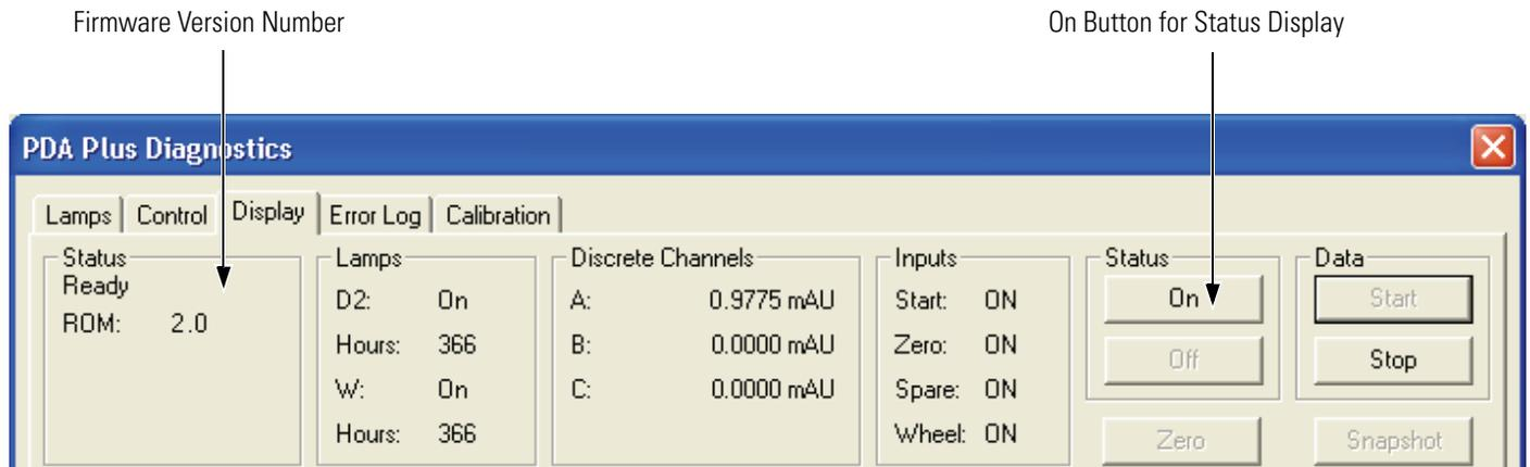
**Figure 45.** PDA Plus Diagnostics dialog box - Display page, showing the firmware version numbers
