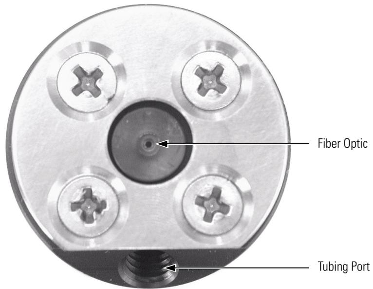
**Figure 5.** End of LightPipe flow cell, showing the sensitive optical fiber
