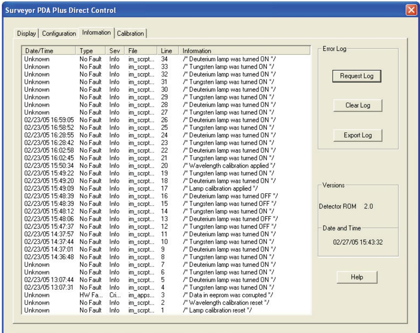
**Figure 66.** Surveyor PDA Plus Direct Control dialog box – Information Page, showing the event log
