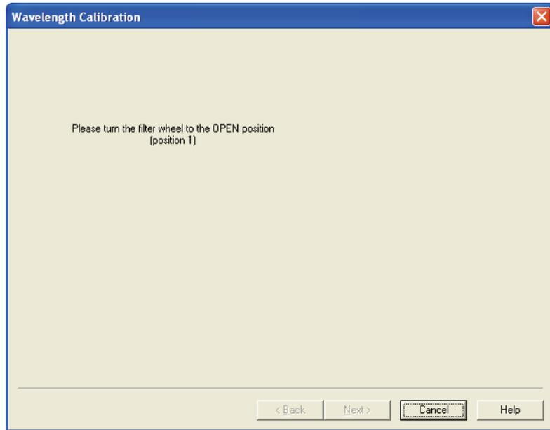
**Figure 52.** Wavelength Calibration wizard – page six, directing you to turn the Holmium Oxide filter wheel back to position 1
