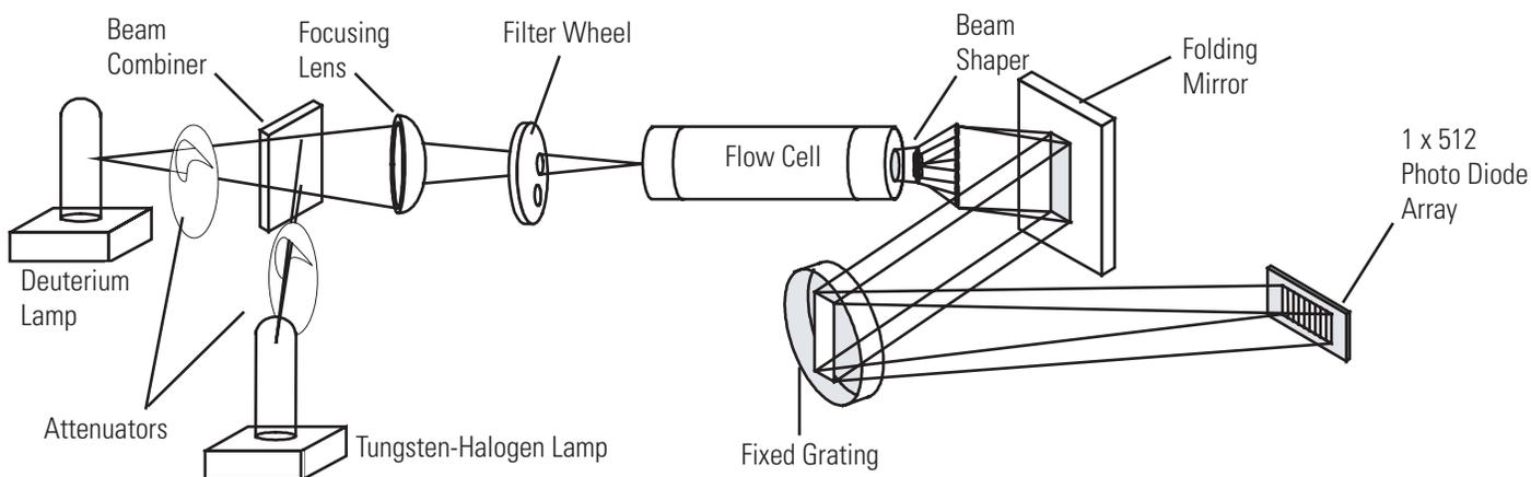
Figure 2. The Surveyor PDA Plus optical system
