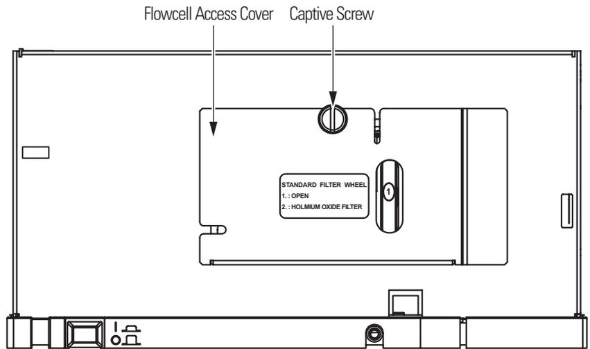
**Figure 78.** Front of Surveyor PDA Plus Detector, with the front doors open
