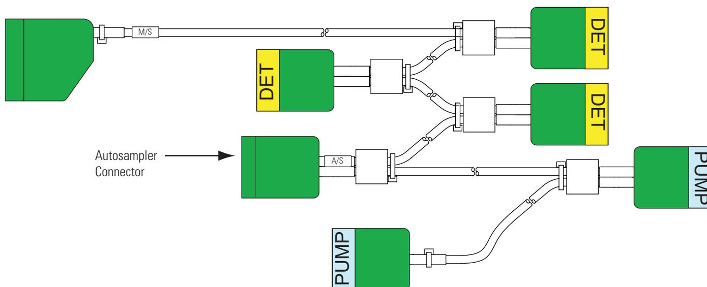
**Figure 9.** Seven-connector version of the system interconnect cable
