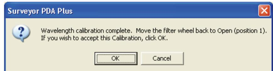
**Figure 34.** Calibration message reminding you to return the filter wheel to position 1
