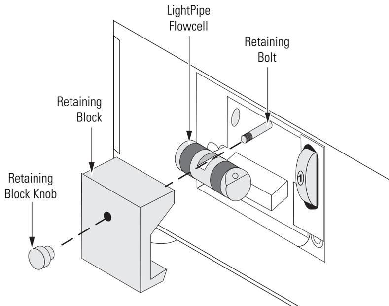
**Figure 79.** Surveyor PDA Plus Detector, showing the removal of the LightPipe flow cell
