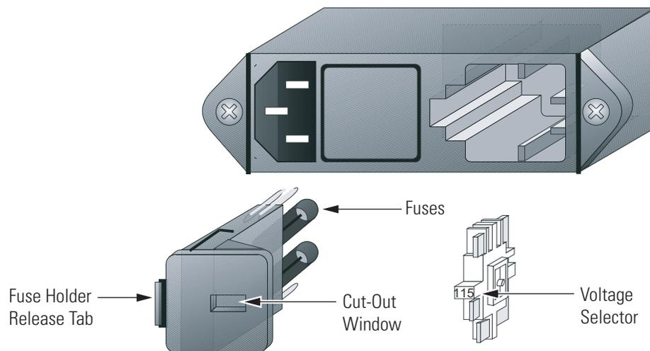
**Figure 7.** Power entry module, showing selection of the proper voltage
