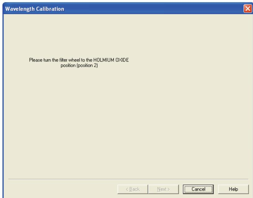
**Figure 50.** Wavelength Calibration wizard – page four, directing you to turn the filter wheel
