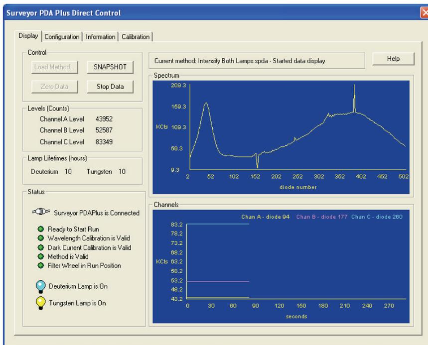
Figure 71. Viewing a scan of the lamp intensities
