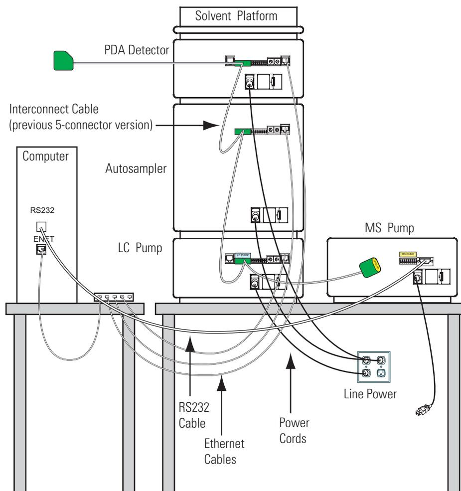
**Figure 8.** Rear panel connections for the Surveyor Plus LC system
