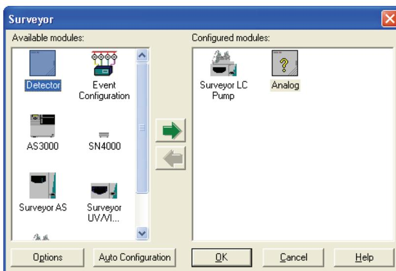
**Figure 22.** Surveyor dialog box, showing the Surveyor LC Pump and the Analog icon added to the Configured modules pane
