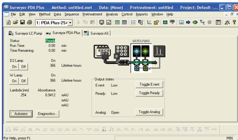
**Figure 28.** ChromQuest Instrument Status window, showing the Surveyor PDA Plus page
