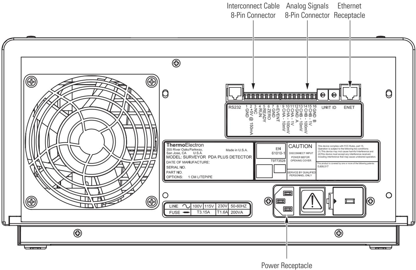
**Figure 10.** Rear panel of Surveyor PDA Plus Detector
