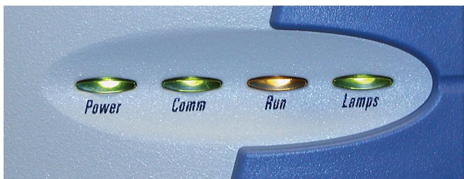
**Figure 3.** Surveyor PDA Plus Detector status LEDs
