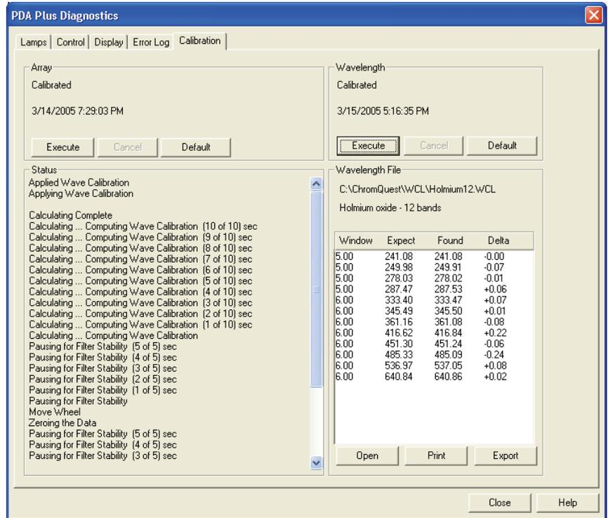
**Figure 35.** Diagnostics dialog box - Calibration page, showing acceptable Delta values
