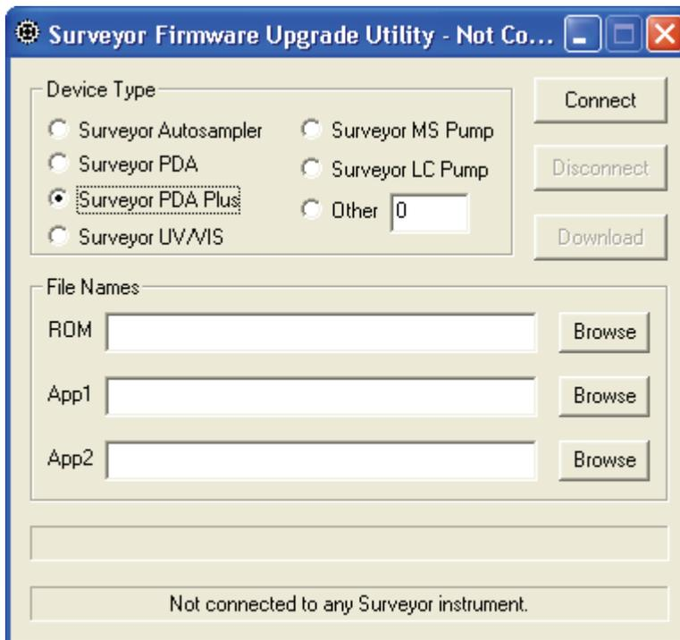
**Figure 85.** Surveyor Firmware Upgrade Utility, showing the Surveyor PDA Plus option selected
