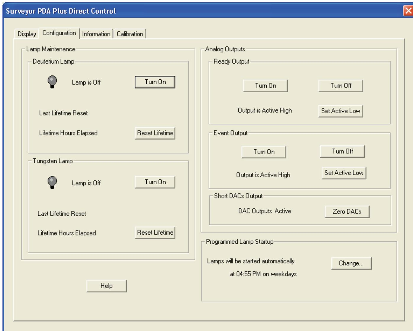
**Figure 18.** Surveyor PDA Plus Direct Control dialog box – Configuration page in Xcalibur
