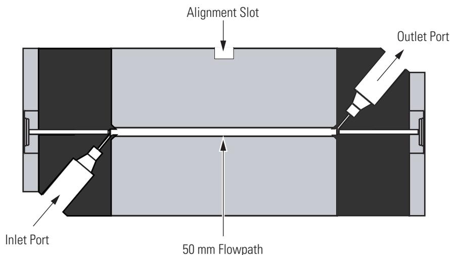
**Figure 4.** Schematic of LightPipe flow cell, showing the internal flow path
