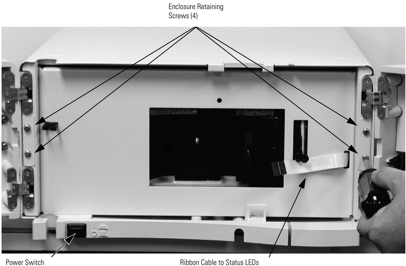
**Figure 80.** Detector with front doors open, showing the enclosure retaining screws and LED ribbon cable
