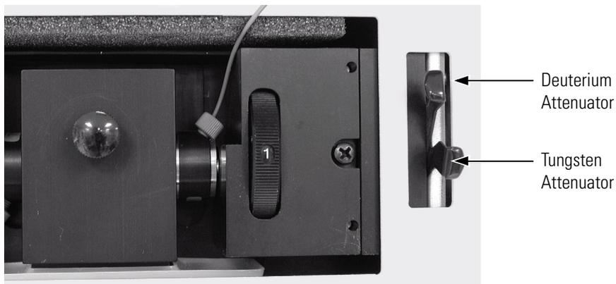
**Figure 44.** Front view of the detector, showing the attenuators
