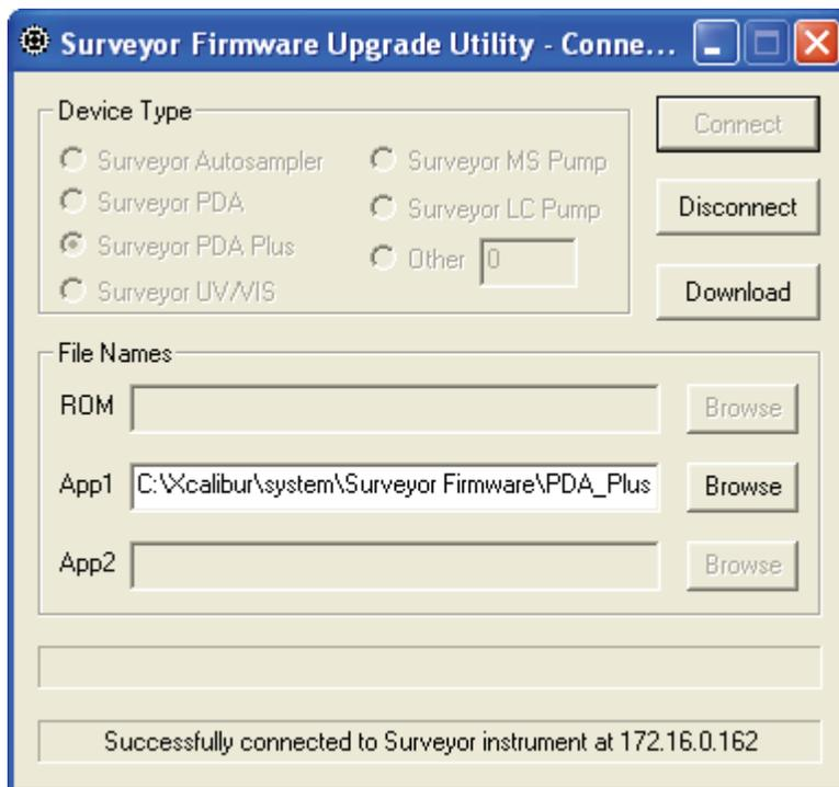
**Figure 86.** Surveyor Firmware Upgrade Utility, showing a successful connection to the Surveyor PDA Plus Detector
