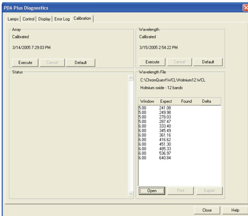
**Figure 31.** Diagnostics dialog box - Calibration page, showing the Holmium12 Wavelength Calibration File selected
