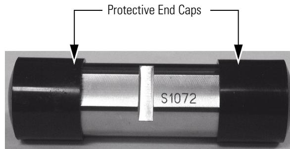
**Figure 15.** LightPipe flow cell with the protective end caps installed
