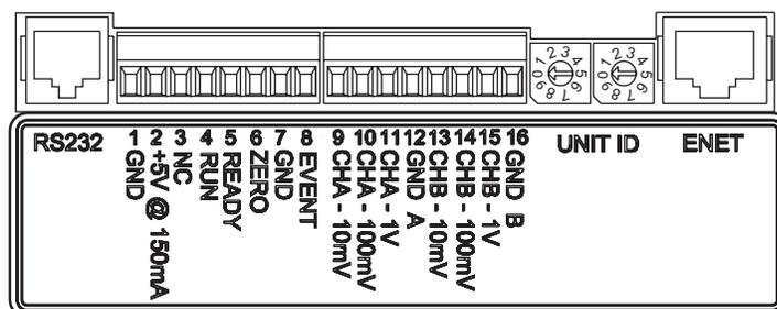
**Figure 11.** Back panel of Surveyor PDA Plus Detector
