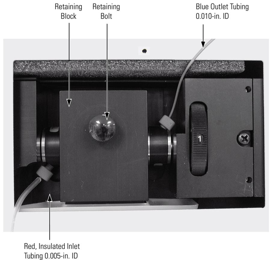
**Figure 16.** Flow cell, showing inlet and outlet tubing connections
