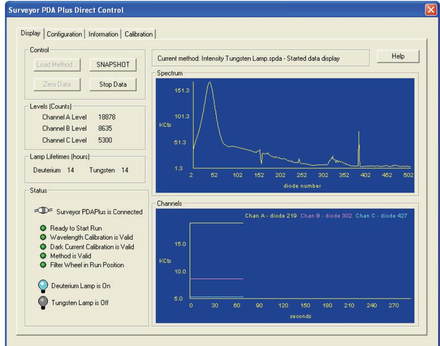
**Figure 72.** Direct Control dialog box – Display page, showing an intensity scan with the deuterium lamp
