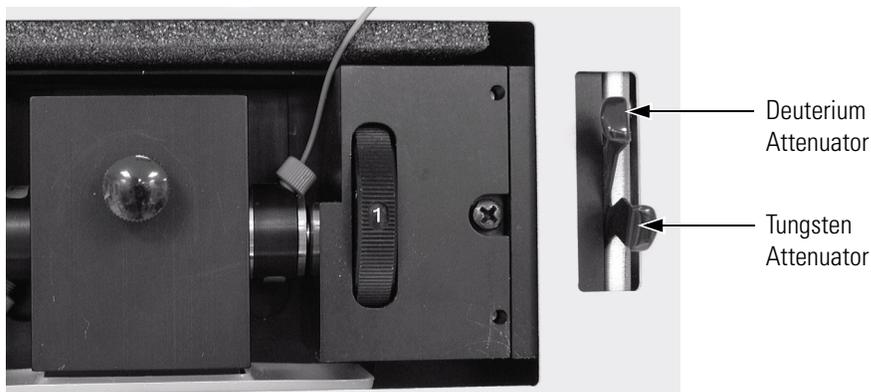
**Figure 75.** Front view of the detector, showing the attenuators
