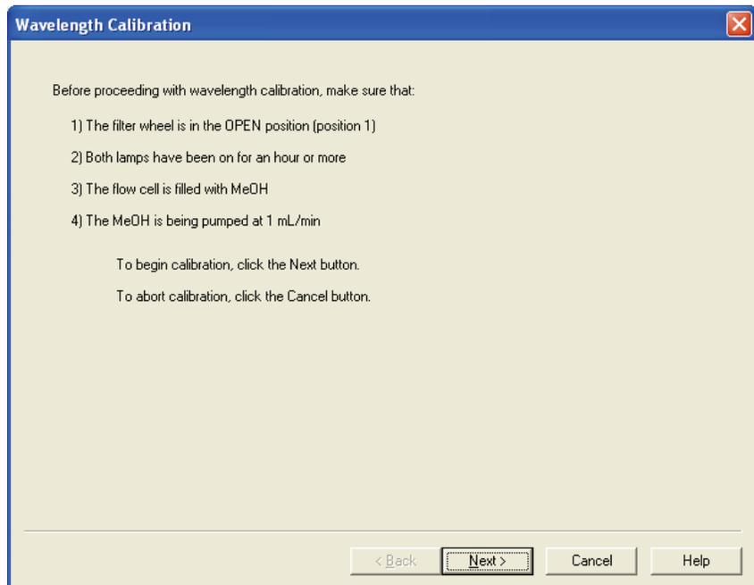
**Figure 47.** Wavelength Calibration wizard – page one, listing required preconditions
