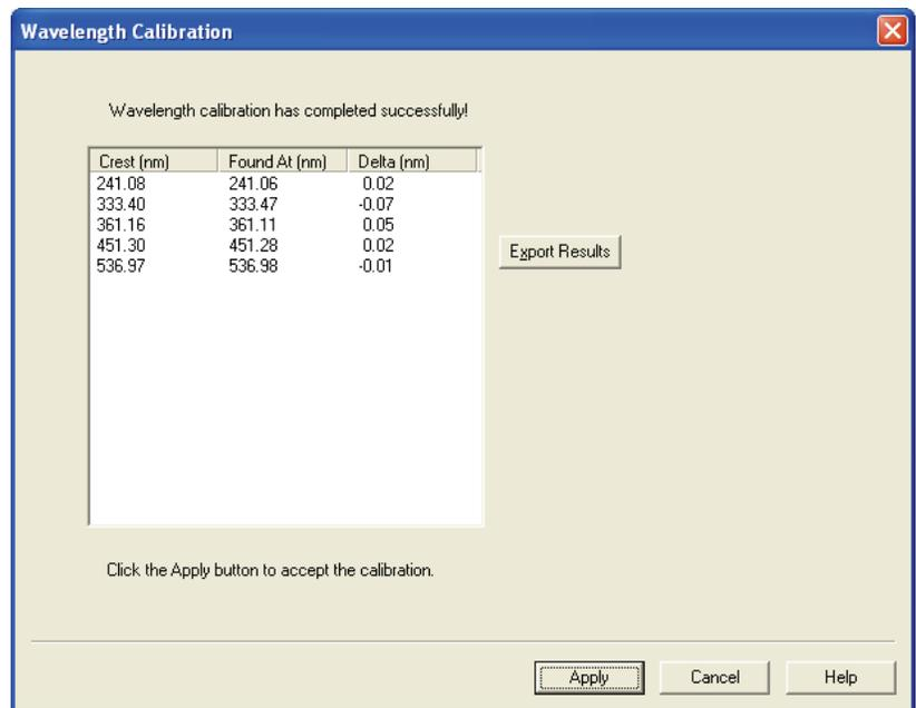
**Figure 54.** Wavelength Calibration wizard – page seven, showing the Delta values
