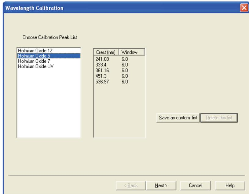
**Figure 48.** Wavelength Calibration wizard – page two, showing a list of calibration files
