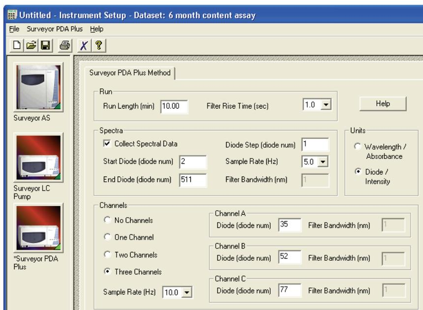
**Figure 69.** Surveyor PDA Plus Method page, showing the selection of the Diodes/Intensity option
