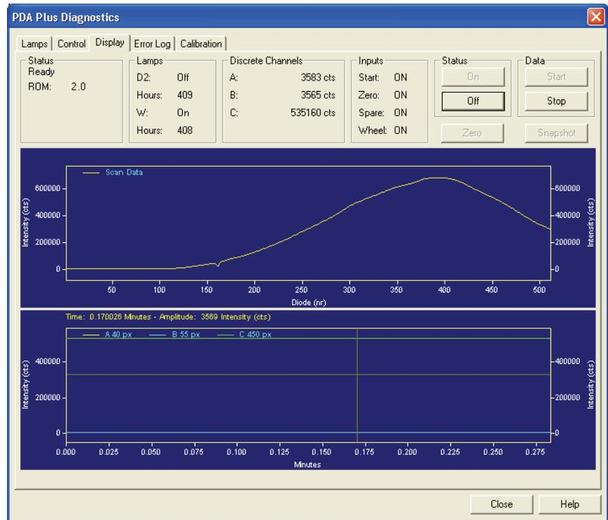
**Figure 41.** PDA Plus Diagnostics dialog box - Display page, showing an intensity scan with just the tungsten lamp
