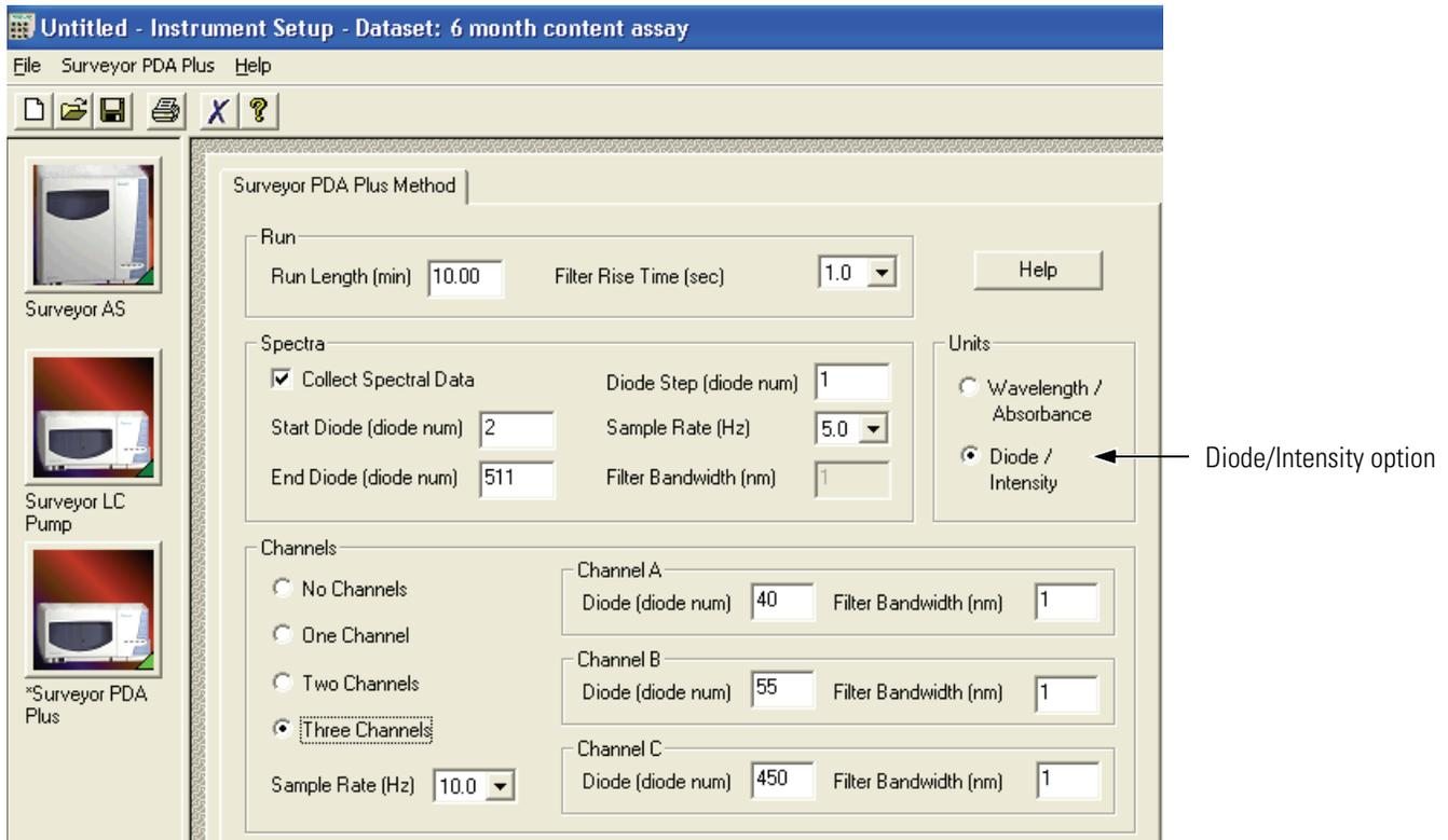
**Figure 67.** Surveyor PDA Plus Method page, showing the selection of the Diodes/Intensity option
