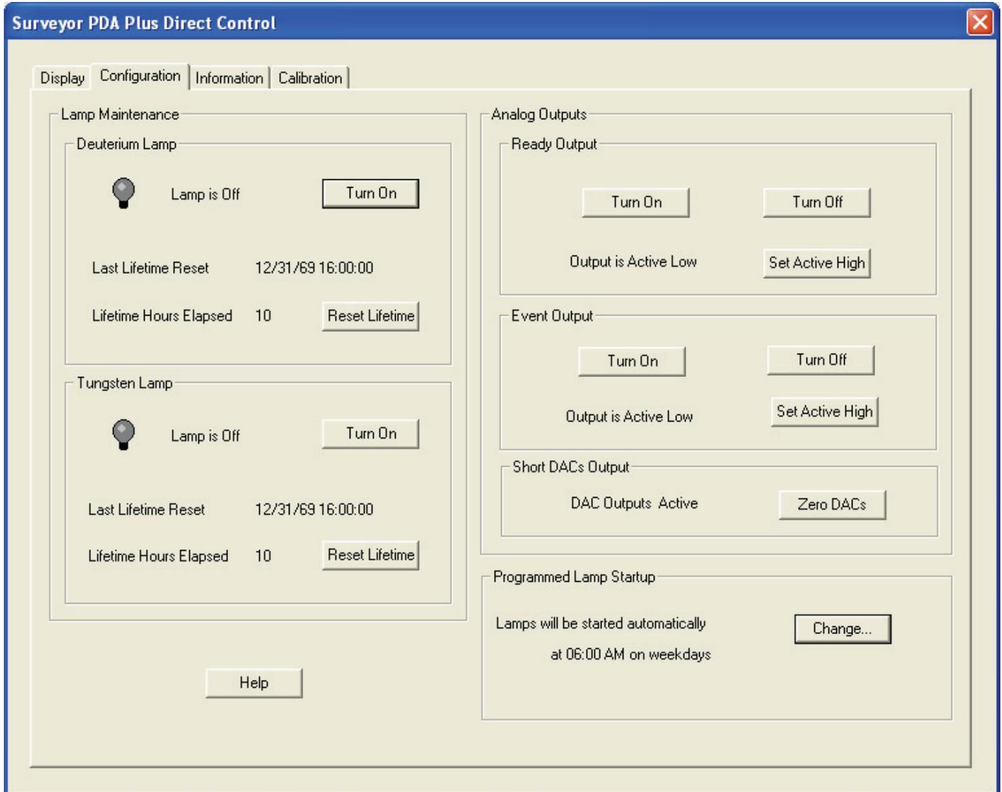
**Figure 73.** Surveyor PDA Plus Direct Control dialog box – Configuration page
