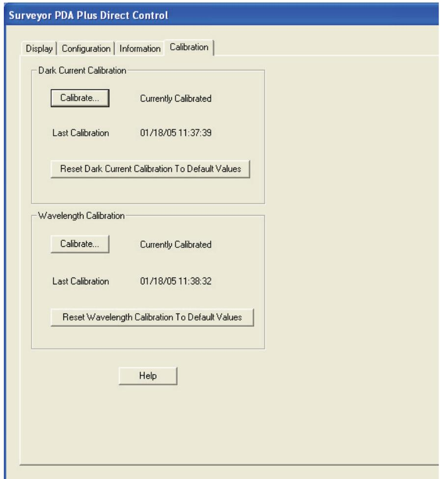
**Figure 65.** Surveyor PDA Plus Direct Control – Calibration page, showing the status as “Currently Calibrated”
