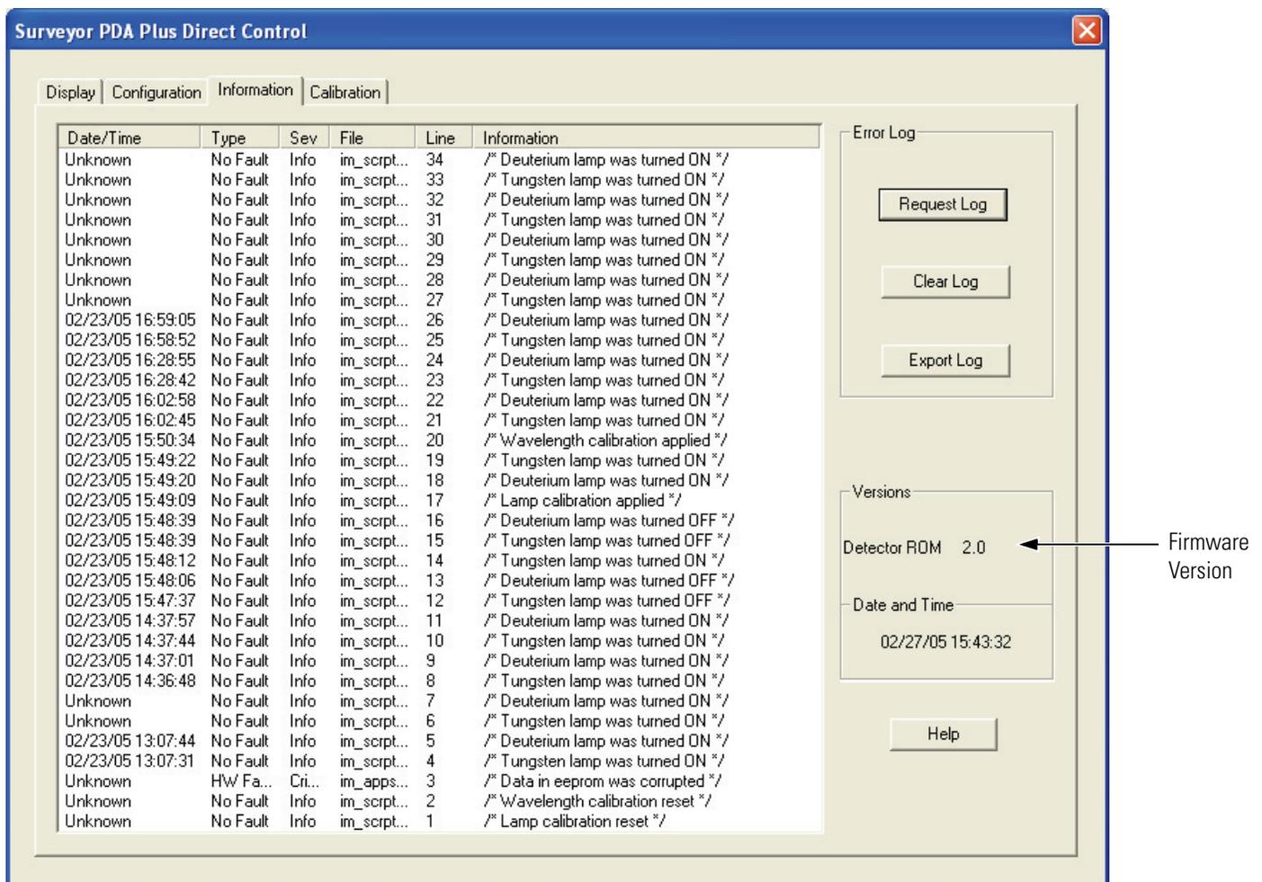
**Figure 77.** Direct Control dialog box - Information page, showing instrument firmware versions in the Versions area
