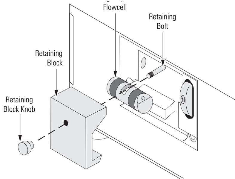
**Figure 14.** Surveyor PDA Plus Detector, showing LightPipe flow cell installation
