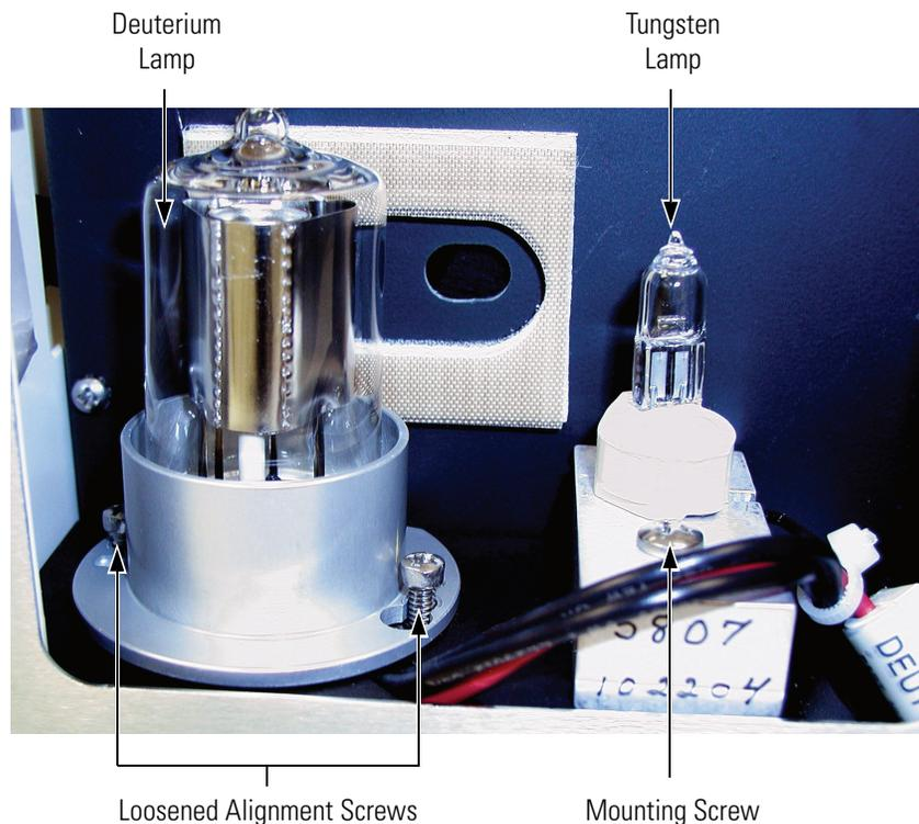
**Figure 83.** View of the deuterium lamp, showing the alignment screws loosened by four turns
