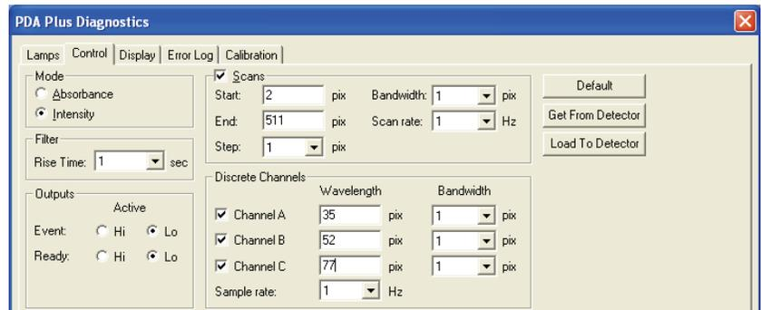
**Figure 38.** PDA Plus Diagnostics dialog box - Control page, showing discrete channels settings
