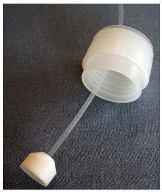
3. Place the solvent reservoir filter and inlet line into the solvent reservoir bottle. Then screw the cap with the stick-on label onto the solvent reservoir bottle until it is secure.
