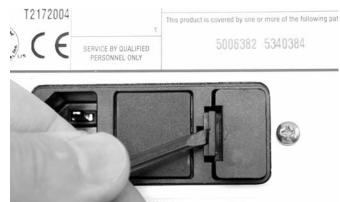
3. Pull out the fuse holder, and remove the fuses (see Figure 75).
