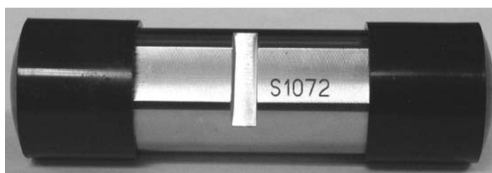
Figure 23. LightPipe flow cell with protective end caps, ready for storage
