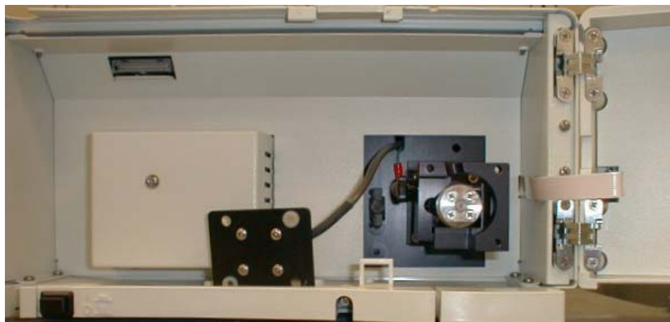
Figure 27. Photodiode mount resting on the detector's drip tray
