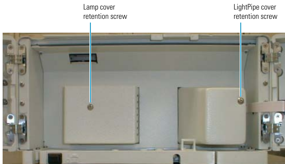
Figure 19. Front panel of the UV/Vis detector with the LightPipe and lamp covers
