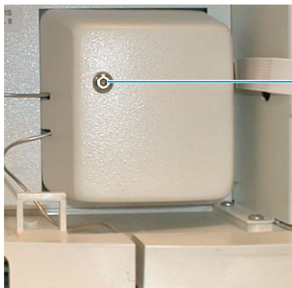
Figure 25. Surveyor UV/Vis Plus Detector with the flow cell cover installed
