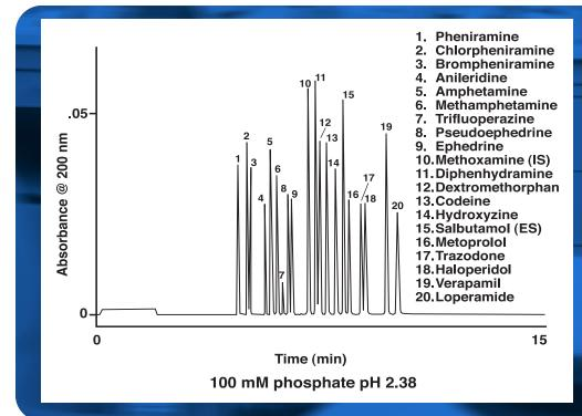
When capillary electrophoresis was introduced, it was seen as a revolutionary technique. Now, it's fulfilling a role as a workhorse in analytical laboratories. In fact, CE should be considered first when dealing with highly polar, charged analytes. It has excelled in the rapid analysis of ions, and become predominant for impurity analysis of basic and chiral pharmaceuticals.
