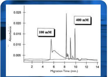
Complex sample matrices require high ionic strength separation buffers for optimum resolution. The P/ACE MDQ's liquid temperature control system allows the use of these buffers without the problems associated with excessive joule heating.
