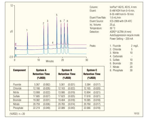
Reagent-Free IC systems produce consistent lab-to-lab eluent concentrations for highly reproducible retention times and peak areas. Results are the same day to day, system to system, and lab to lab.
